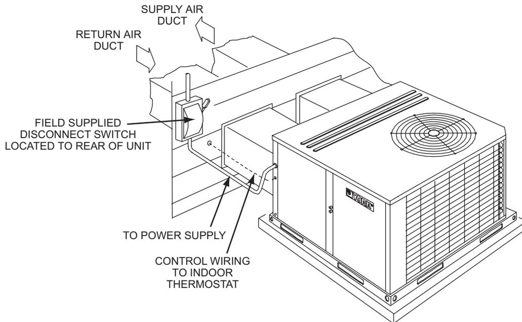
**Unit Typical Roof Curb Installation**
