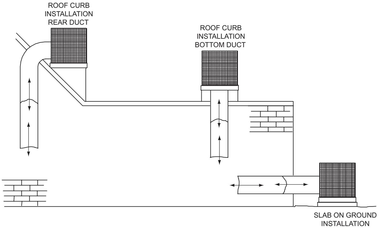
**Unit Typical Slab on Ground Installation**
